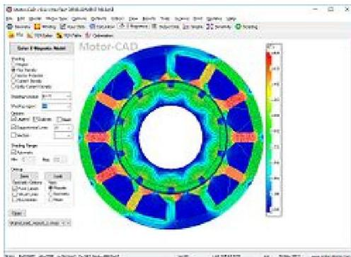
Motor-CAD electromagnetic results
