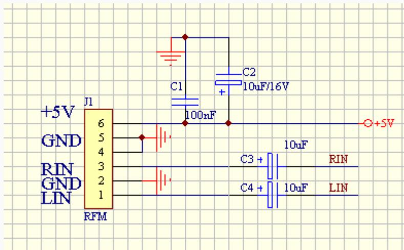
For the audio input and output of the module, need to connect to a capacitor of 10uF, and then weld wires or stereo plug wire. Supply 5V DC power supply to modules, or use 3xAA batteries. If the power supply is from 5V switching power supply, need to add decoupling capacitor 100uF, it is best to connect a inductor in series to the positive pole.
