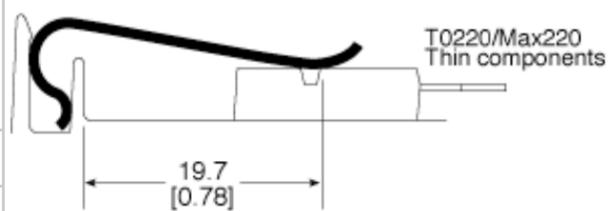
**Force:** 40 N [9.0 lbs]**Width:** 12 mm [0.47 in]**Thickness:** 0.6 mm [0.02 in]**Part Number: MAX12NG**
